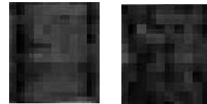
Figure 2: Maps of fractional anisotropy obtained within the capillary packing with STE preparation and \Delta of 115 ms (left) and 1915 ms (right). The averaged anisotropy decreases with diffusion time.
