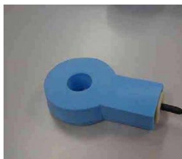
Figure.1 Receive only small surface coil used for high spatial resolution diffusion study.
