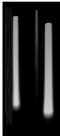
Fig. 2 Maximum intensity projection of the 3D-dose distribution originating from 3 pencil beams at diameter: d_1=2.1 , d_3=0.86 , d_2=1.5 mm.
