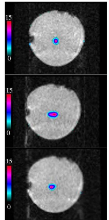
Figure 2: Snapshot of the temperature distribution after 200s of heating for the static experiment (top), under motion, but without compensation (middle) and under motion with applied motion compensation (bottom).
