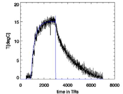
Figure 1: Target temperature profile (blue) and measured temperature (black) at the hot-spot of the motion compensated heating experiment.
