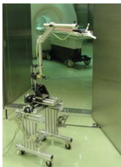
Fig. 1 A motorized robot to assist MR-guided microwave ablation of liver tumors.
