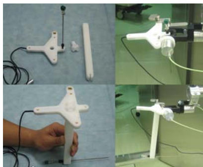
Fig. 2 A new robot hand-piece with a detachable longitudinal pole. Punctures in both vertical and horizontal directions are available.
