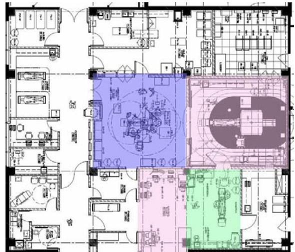
Figure 1: MR-OR suite layout including surgical (blue), MR (pink), and anesthesia (green) areas.
