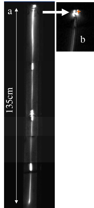
Fig.2: Phantom images: a.) RF-safe visualization of the entire catheter. b.) Active Tracking
