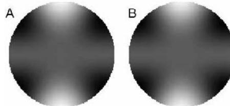
**Figure.** Real part of the x-component (y-axis is vertical) of the magnetic field in the  $z = 0$  plane. A: the target field  $\mathbf{H}_{43}^E$ ; B: the field generated by the array coil. The field is zero at the center where the image intensity is grey, and the black areas have negative values.
