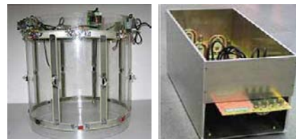
Fig 1: The constructed DBC coil and Butler matrix
