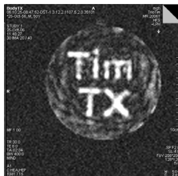
Fig 2: parallel excitation with the body coil and receiving with the 12 channel head matrix coil, spiral trajectory with 4x acceleration
