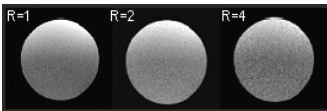
Figure 4, Transverse image of a phantom (4.7g /mol NaCl) with SENSE reconstruction for different acceleration factors.
