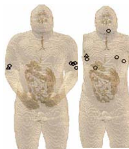
Figure 2: Positions of the peak SARs before (quadrature) (Δ) and after (o) optimization over 5 84-mm slabs (3axial/1 coronal/1sagittal) with (left) and without (right) the arms included in the optimizations.
