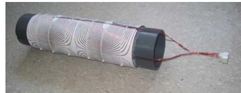
Figure 2: The gradient coil constructed for use in the field-cycled MRI scanner.
