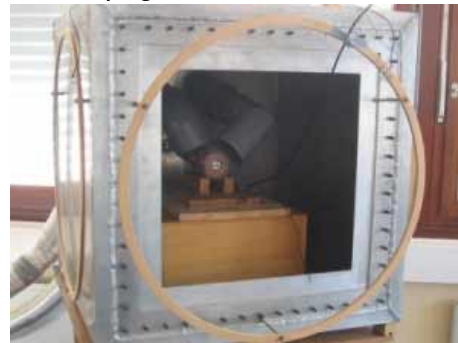
Fig. 1 The Earth Field NMR device with shims, shielding and air-cooling.
