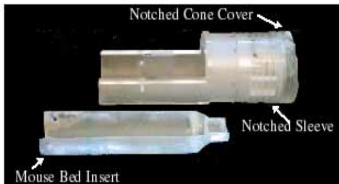
Figure 1: Photograph of constructed passive shim assembly.
