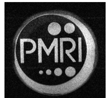
Figure 3: Image of acrylic-cutout phantom in water, acquired using the Medusa Console (Figure 1) on the Stanford PMRI scanner.
