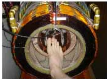
Figure 1 (left) Photo of 0.4T/0.06T Prepolarized MRI knee scanner. (Right) Timing diagram for Prepolarized MRI scan.
