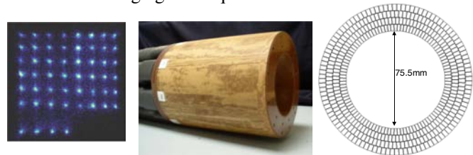
Figure 2: From left to right 2D coincidence flood position histogram, PET front end housed in Tufnol material, Crystal configuration side
