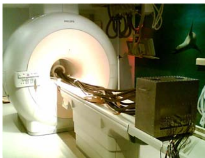
Figure 3: PET scanner inside the Philips Achieva 1.5T MR scanner
