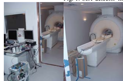
Fig. 2: Photograph of the single-module CZT setup that was used in the 3 T imaging experiments
