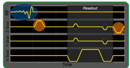
Figure 2. Fe-SSFP pulse sequence. A spectrally selective RF pulse (blue oval) suppresses on-resonant signal. Rephasing gradients (orange circles) counteract the local gradient present near the dipole marker and spoil background signal.
