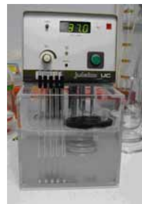
Figure 1. The water-bath containing tubes with cell suspensions.
