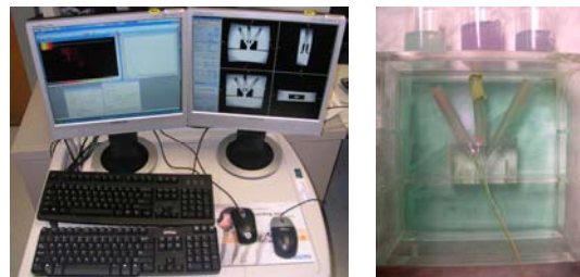
Figure 2: (a) Interactive setup for simultaneous control of the EES (left) and MRI (right). A projector also permitted control of the MR system from within the scan room. (b) Vascular phantom loaded with three differently-doped agar gels.
