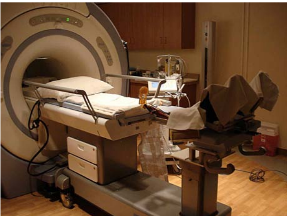
Figure 1: Picture of the custom imaging table for patient positioning in the supine position docked to GE 1.5 T MRI scanner.
