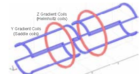
Figure 6. Y and Z Gradient coils capable of 2D steering of the heating
