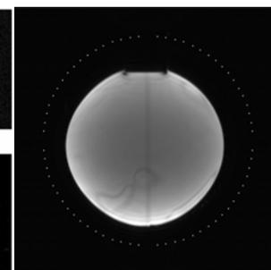
Fig 3: <sup>1</sup>H Proton density weighted images of a 17.8 cm spherical saline phantom at acquired at 7 T
