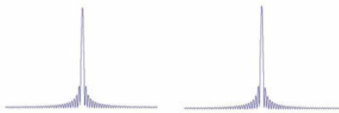
Fig. 2 PSF of (right) rectangular, (left) circular k-space 3D GRASE
