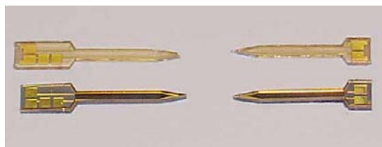
Figure 2 Photograph of the older silicon-based needles (lower) and the new all plastic ones (upper).
