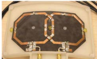
Fig. 1: Dual array for proton imaging at 3.0 T; note vitamin cap fiducials (yellow lozenges).
