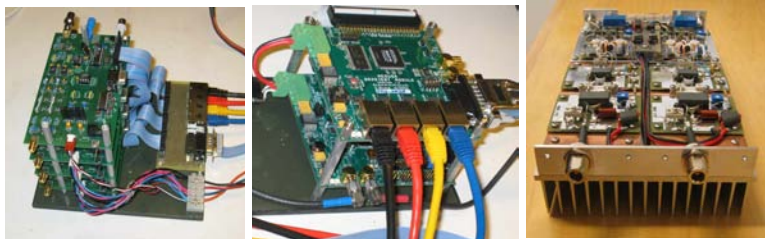
Figure 1: Left: An array of 4 vector modulators provide 4 output channels. Center: A 4 channel high speed digital output system with USB interface, controller and single channel digital synthesizer and digital receiver. Right: Dual channel 300W RF amplifier stage.
