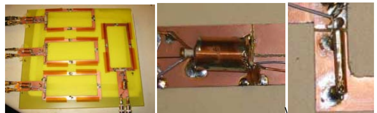
Figure 2: 4 coil transmit array with close-up showing bifilar balun and RF current transducer.
