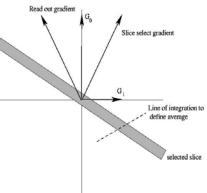
Figure 2: Slice selection and averaging in slant-slice imaging.
