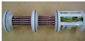
Fig.1. The homebuilt gradient system
