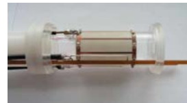
Fig.2 The homebuilt high-pass birdcage coil
