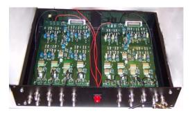
The MCC is driven by two Labview-controlled National Instruments Analog Output Cards in a peripheral PC, which is controlled by the MRI console using network communication protocol. Adjustments are possible with 16-bit precision over both a range of 0-200 degrees phase shift and 0-20dB attenuation. The MCC was calibrated before use in the MRI scanner system using an Agilent 4395A network analyzer. For each control voltage, the resulting output signals were stored in a look-up table.
