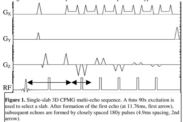
**Figure 1.** Single-slab 3D CPMG multi-echo sequence. A 6ms 90x excitation is used to select a slab. After formation of the first echo (at 11.76ms, first arrow), subsequent echoes are formed by closely spaced 180y pulses (4.9ms spacing, 2nd arrow).
