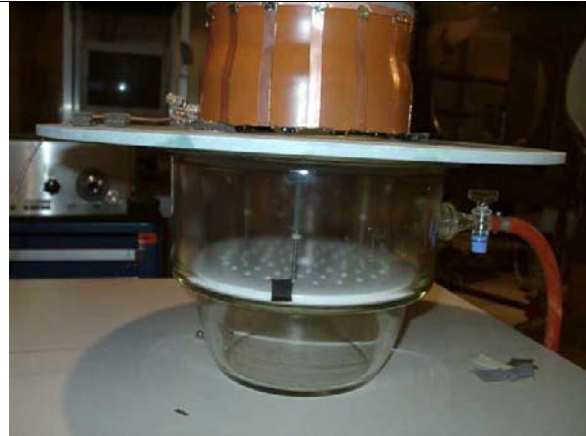
Fig. 2: The test setup (RF-shield in vacuum, coil outside)
