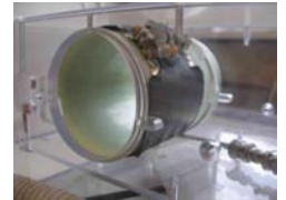
Fig. 1: Solenoid RF-coil using strip conductors fixed on a fiberglass cylinder.
