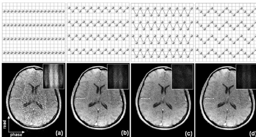
**Figure 2:** GRAPPA reconstructions after accelerated (R=4) (a) conventional sampling and various zig-zag sampling trajectories (b,c,d). In the right corner the difference to the fully encoded reference image is given in each case.
