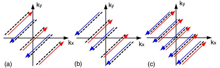
Fig. 1. In oblique EPI scans with asymmetric gradient delays, acquired raw data represent samples on the red and blue lines, not on the intended dashed black lines (a): odd frame. (b): even frame. (c): When (a) and (b) are combined, the blue lines become uniformly spaced with 1/FOV interval along logical phase-encoding direction, and so forth for the red lines.
