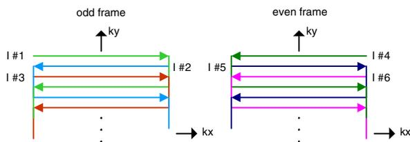
Fig. 3. Double-alternating EPI trajectory used in cardiac study. The interleaf order is shown.
