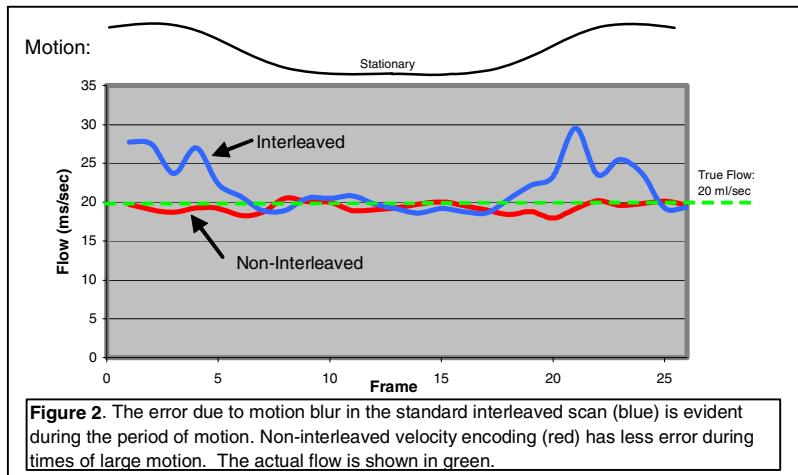
**Figure 2.** The error due to motion blur in the standard interleaved scan (blue) is evident during the period of motion. Non-interleaved velocity encoding (red) has less error during times of large motion. The actual flow is shown in green.
