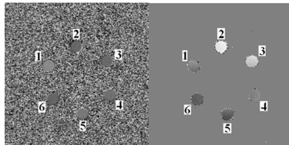
**Figure 1.**  $R_2^*$  (a) and  $\Delta\phi$  (b) susceptibility-weighted images of 5 0.08% agar phantoms serially-diluted with iron (vials 1-5, in decreasing order) and one 0.08% agar phantom (vial 6). The images were calculated between the lowest two TE images for both methods.
