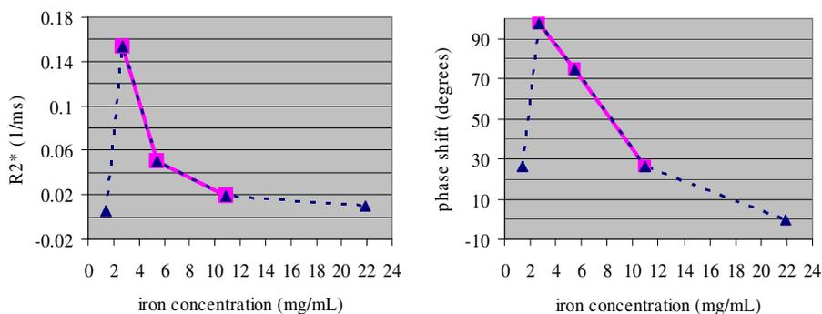
**Figure 2.**  $R_2^*$  (a) and  $\Delta\phi$  (b) versus iron concentration. On both plots, the signals are not reliable due to saturation at the highest concentration and low sensitivity at the lowest concentration. The reliable portion for the curve (solid line) for  $R_2^*$  appears non-linear while  $\Delta\phi$  appears linear to iron concentration.
