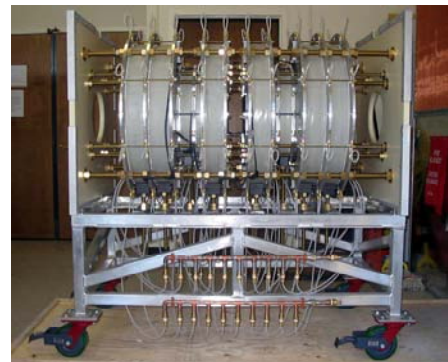
Figure 3: A photograph of the main magnets of the field-cycled MRI scanner. The polarizing magnet is concentric and interior to the readout magnet.
