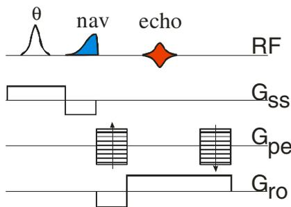
**Figure 1:** Flash sequence with in-slice navigator echo (nav). RF: RF-channel (RF pulse ( $\theta$ ) and image echo (echo));  $G_{ss}$ : slice-selection gradient;  $G_{pe}$ : phase encoding gradient;  $G_{ro}$ : readout gradient.
