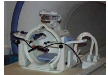
Figure 1. 3T CASL coil configuration.
