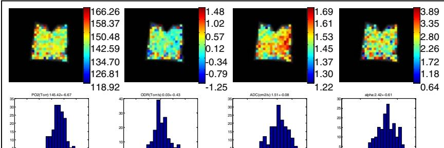
Fig.2. Phantom experiment results:  $PO_2 = 145.42 \pm 6.67$  Torr;  $ODR = 0.03 \pm 0.43$  Torr/s;  $ADC = 1.51 \pm 0.08 \text{cm}^2/\text{s}$ ;  $\alpha = 2.42 \pm 0.61$ ;
