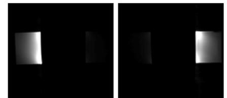
Figure 5 Isolation property of the micro-strip coil. Images are from left and right coils respectively. Aliasing ghost is <1%.
