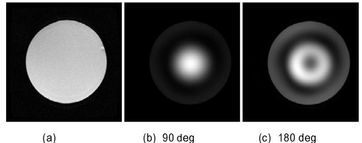
Fig. 4. Gradient echo images of (a) Si phantom, (b) & (c) water phantom.
