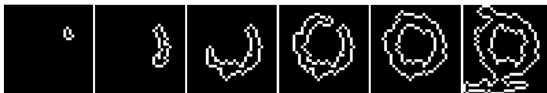
Figure 1. Progression of the guided flood-fill operation using the quality map in Figure 2(c). The calculation intervals are arbitrary.
