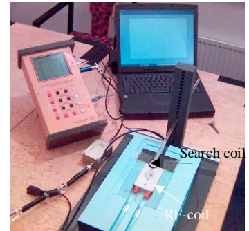
Fig. 2. The experimental setup used for mapping of the B_1 -field.
