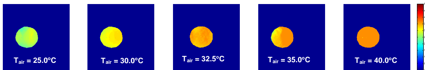
Figure 1. Temperature maps of a phantom containing 1 ml, 10 mM EuDOTA-4AmC in water at pH 7.0. The temperature of the air flowing over the sample are indicated in each figure while those reported by imaging are shown by the color bars.
