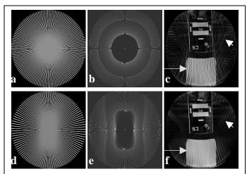
**Figure 1.** Two alignments of the projections: uniform distribution (a), elliptical distribution (d), as well as their point spread functions (b, e), and phantom images (c, f). The streak artifact is significantly reduced along S/I direction (long arrow), but enhanced a little bit along R/L direction (short arrow) due to the elliptical alignment of the projections.
